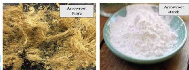
Fig. 1 Arrowroot fiber obtained from starch extraction mill [11].
