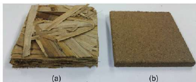
Figure 1: (a) Binderless composite made from rice straw whole particles (b) Binderless composite made from rice straw whole powder [4]
