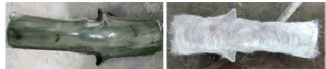
Fig. 3 Natural fiber fabricated Motorcycle Mudguard [4]
